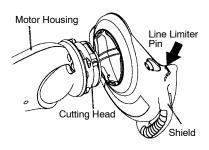
2. Align the installation arrow on the shield with the installation arrow on the motor housing as shown.
